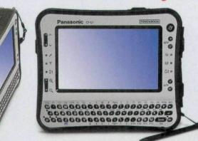
The Panasonic Toughbook U1 comes with a solid-state drive, 1GB of memory and the Intel Atom Processor Z520. It's rated to survive a four-foot drop and has a sealed, all-weather design. It also features integrated Wi-Fi, a backlit QWERTY keyboard, USB and SD card slots, and a 5.6-in. WSVGA sunlight-viewable touch screen.
